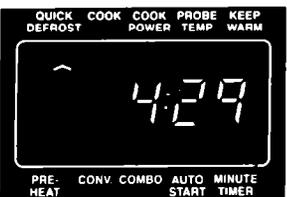
When you touch **START**, the **QUICK DEFROST** Indicator Light will stay on. All other Indicator Lights will go off. The Display counts down the time to show how much time is left in the defrost cycle.
